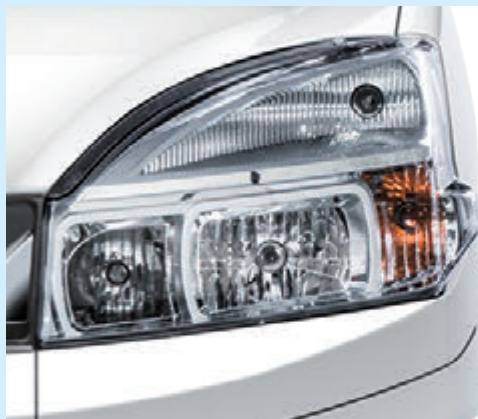
Two-Layer Headlamp With Daytime Running Lamp
